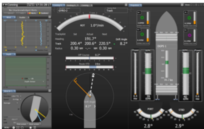
Figure 5 - Drift Test results from Regal Princess
